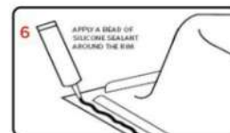
With sink in the upside down position, place a continuous and generous bead of silicone sealant around the entire perimeter of the rim. This serves as a watertight seal.
